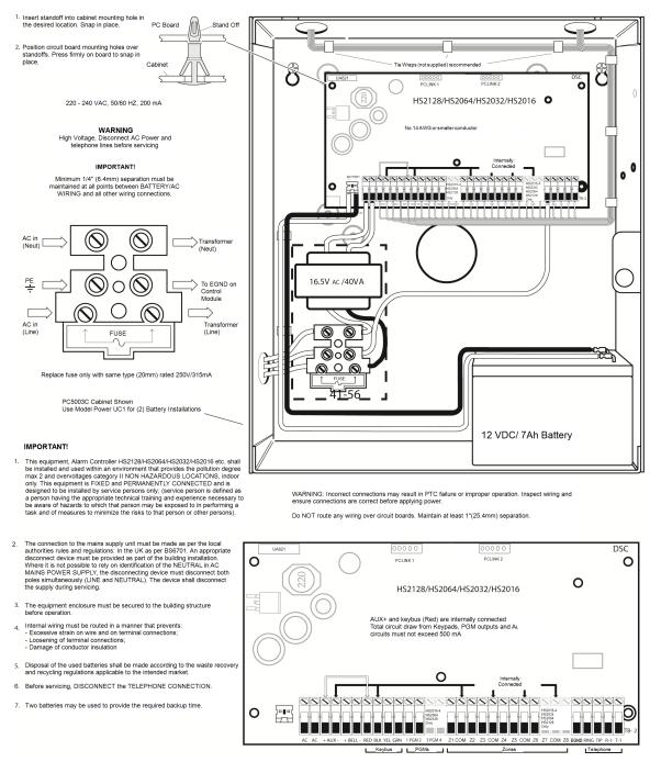
Figure 2-2 Wiring Routing (EN50131 only)
