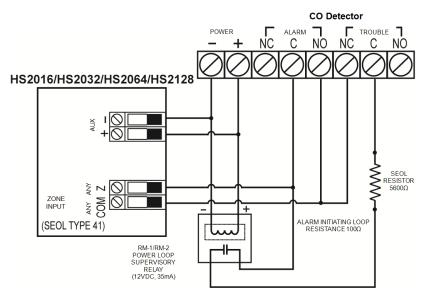
Figure 2-17 CO Detector Wiring
