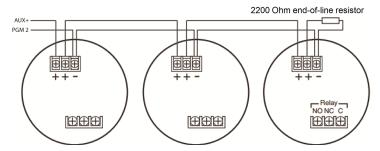
Figure 2-16 2-Wire Smoke Detector Wiring
