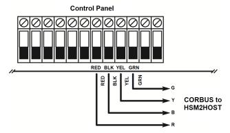
Figure 2-6 HSM2HOSTx Wiring Diagram
