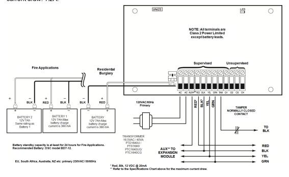
Figure 2-7 Power Supply Wiring
