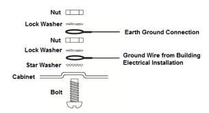
Figure 2-18 Ground Installation
