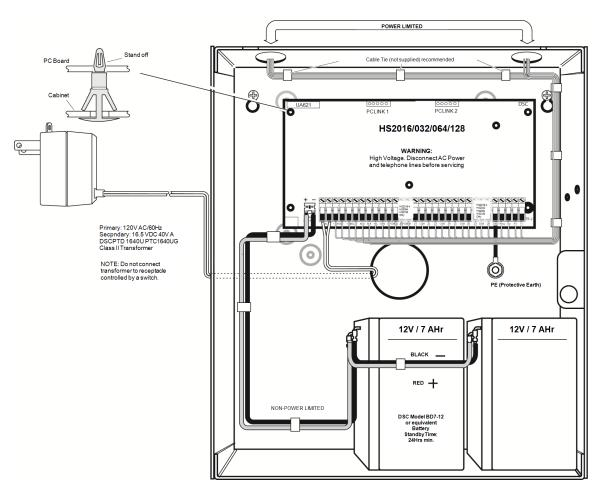
Figure 2-1 Wiring Routing (North America only)
