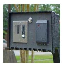
indicate access-granted by the host. The beeper can be used as an alarm that prevents further card reads until the alarm condition is cleared. The "hold" circuit delays code transmission from the reader until the host requests it.
