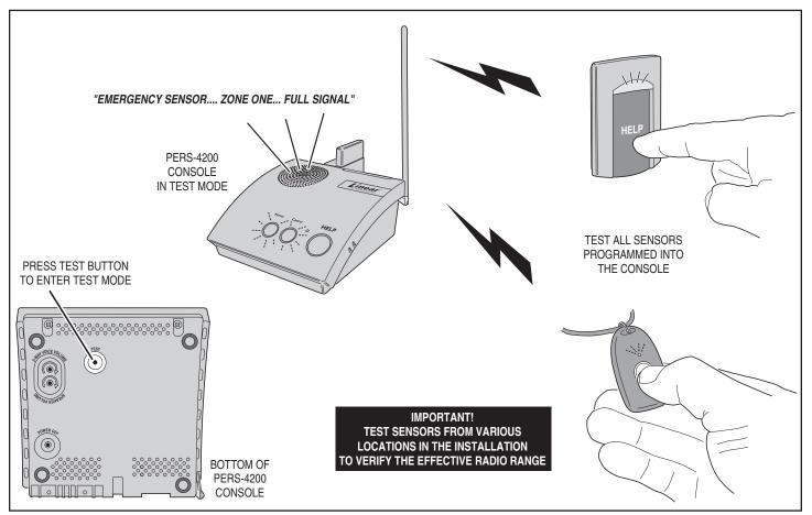
Testing System Sensors
